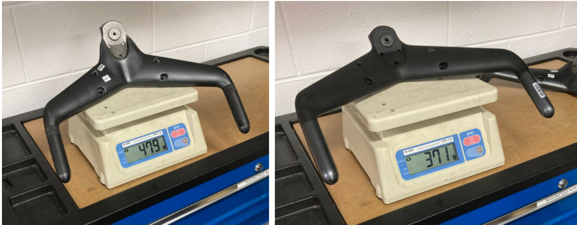
Figure 11 - Bastion (L) vs. Argon standard (R) base bar weights
