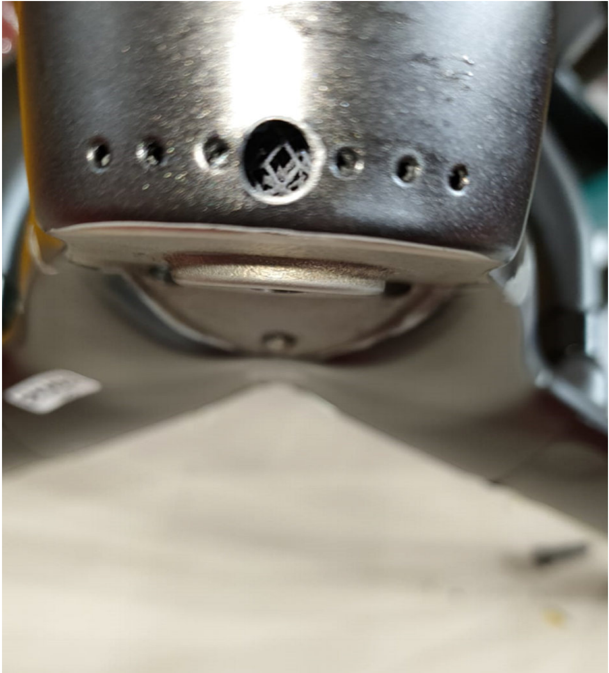
Figure 25 - Bar #3 oxidation inspection hole
