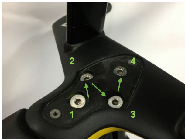
Figure 32: Correct fastening order of pursuit basebar bolts.
