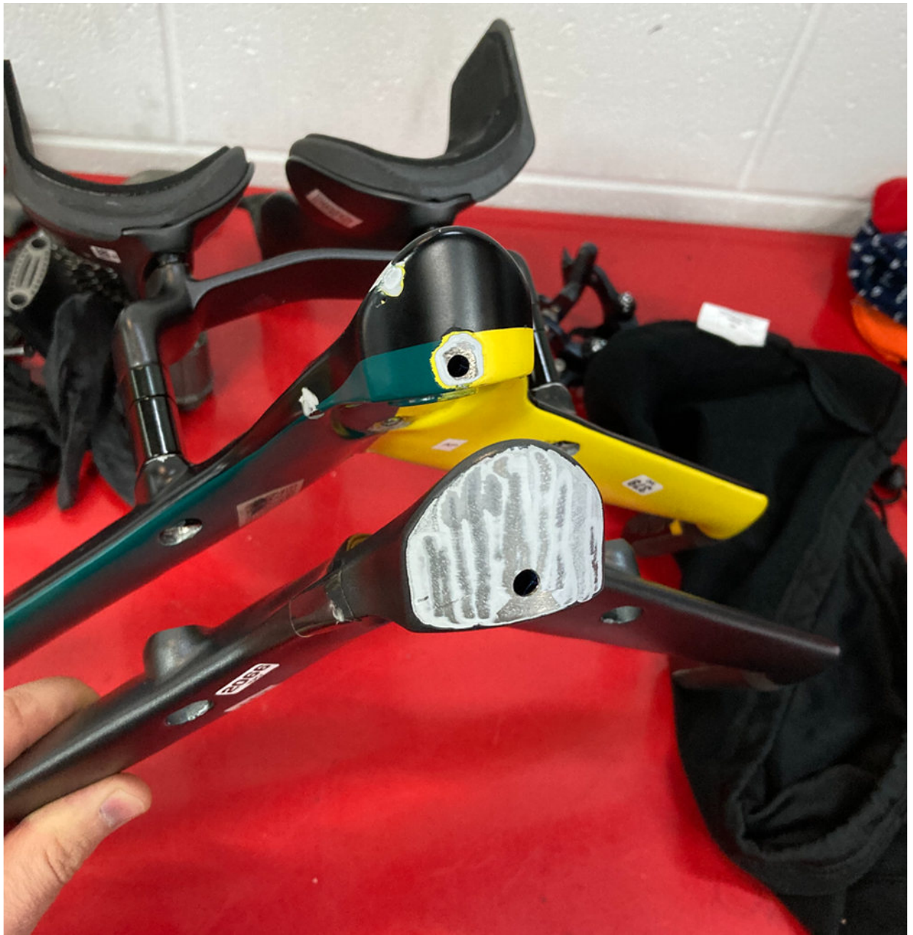
Figure 9 - Bars #1 (top) and #2 (bottom) showing rear surface, no breather holes. Inspection holes drilled by ACT after Tokyo qualifying incident to confirm oxidisation
