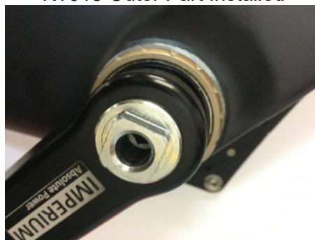
Figure 21: Extracting Imperium crankarm using Cannondale KT013
