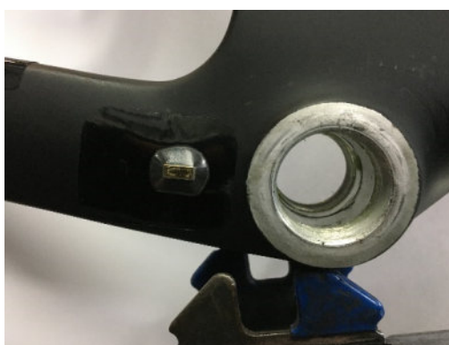
Figure 6: Correctly positioned SRM Magnet.
