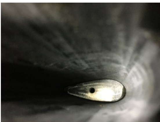
Figure 23: Correctly installed Seat Tube Plug in 2020 Frameset
