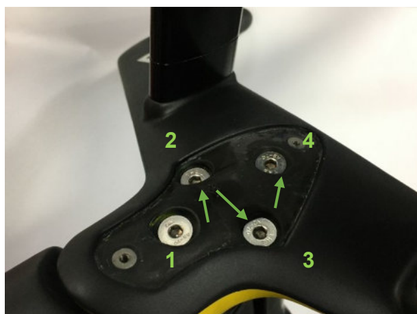
Figure 47: Correct fastening order of integrated sprint bar bolts.
