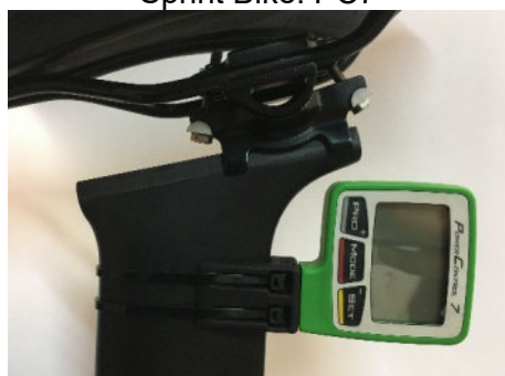
Figure 52: Correct SRM Mount Orientation, NDS View
