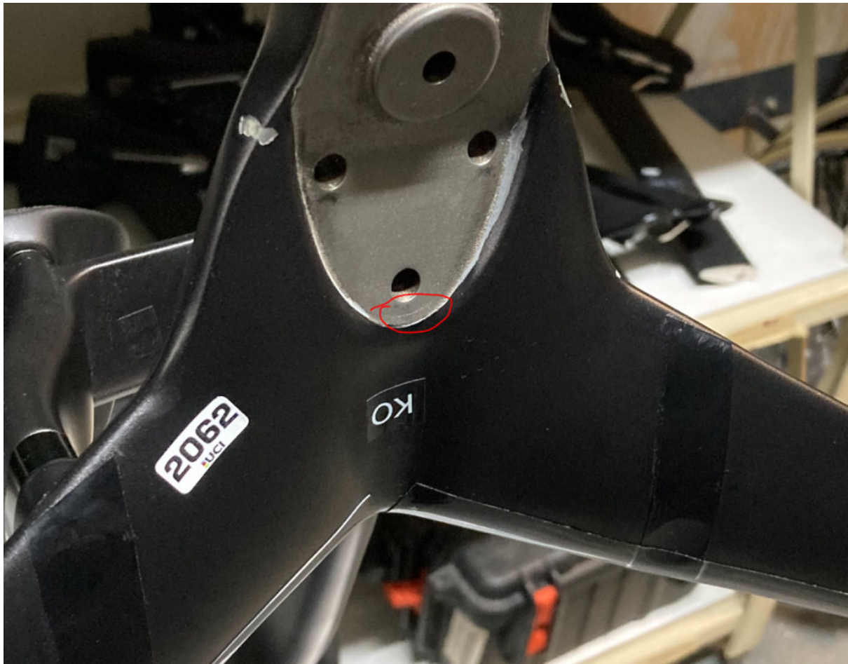
Figure 24 - Apparent crack beginning to form at same location on bar #3
