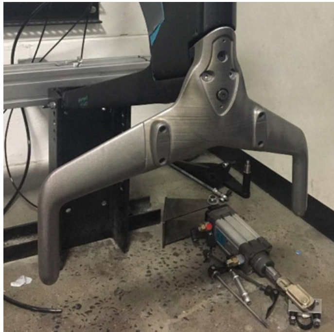
Figure 6: Base Bar CA-06 mounted in the Test Rig
