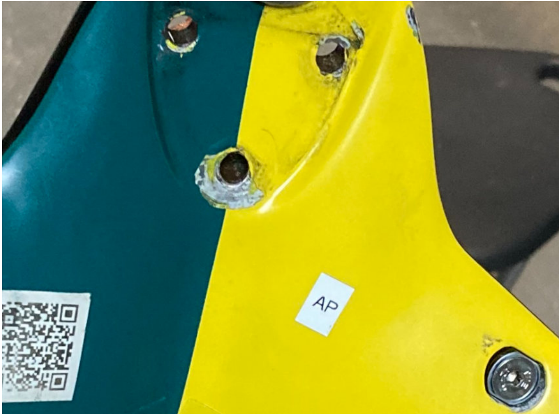
Figure 18 - Closeup of paint worn away on bar #1
