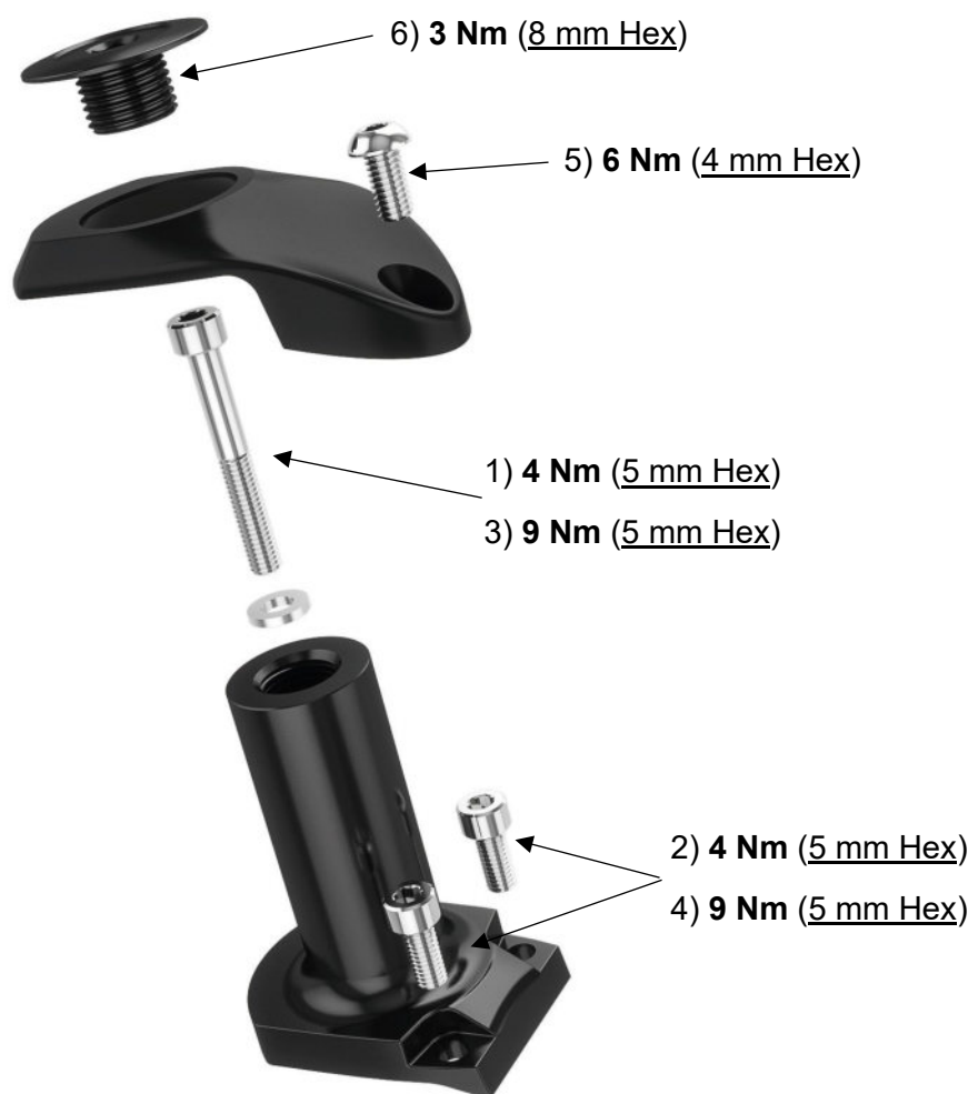
Figure 50: Steerer Module Assembly Order
