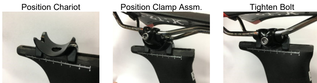
Figure 27: 2020 Seat Clamp Assembly Steps
