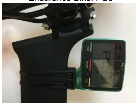
Figure 52: Correct SRM Mount Orientation, NDS View
