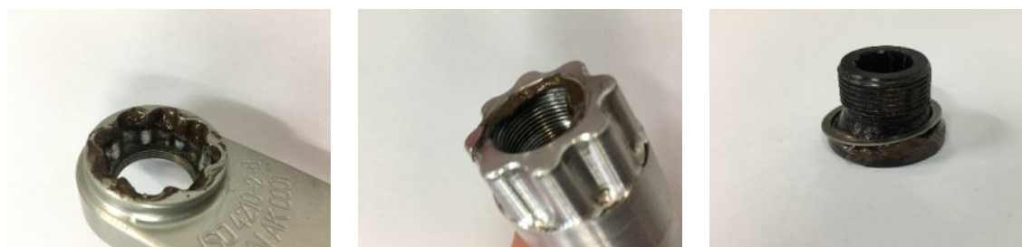
Figure 19: Correct application of copper anti-seize for Imperium crank.
