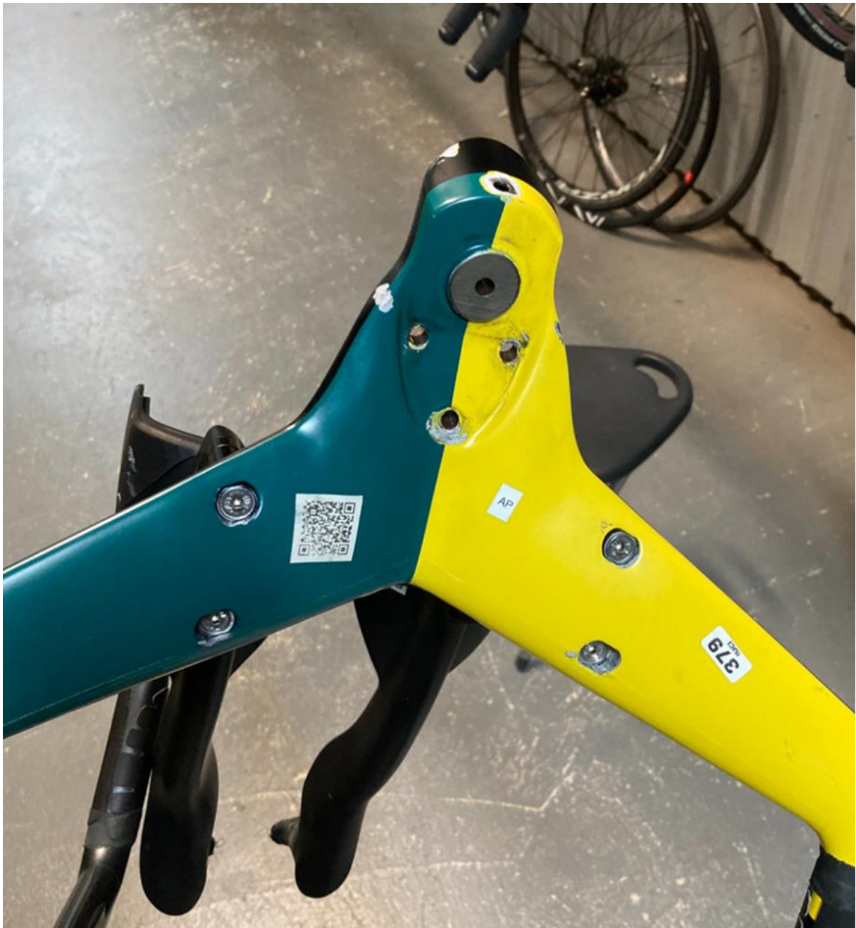
Figure 14: Number One Base Bar with paint missing from the front bolt hole
