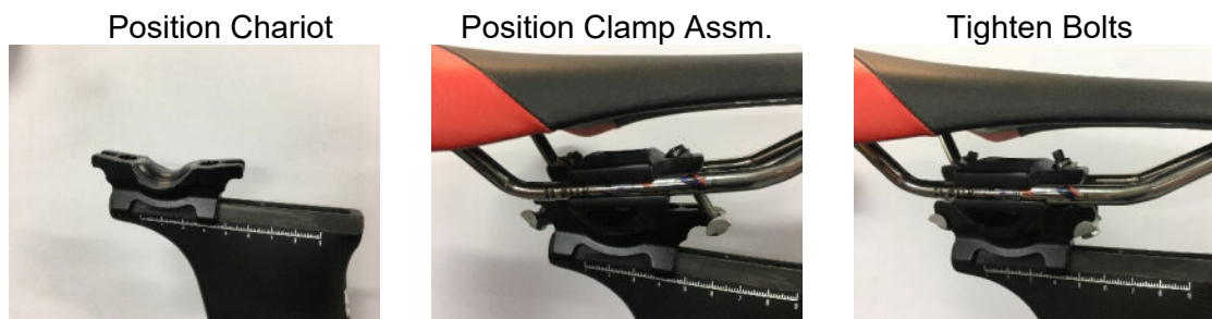
Figure 25: 2018 Seat Clamp Assembly Steps
