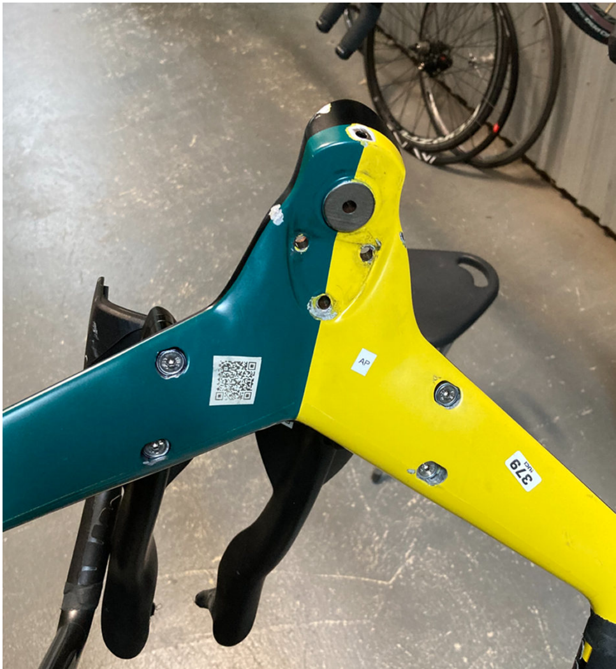
Figure 17 - Bar #1 - original, delivered in 2019. Painted underside to match livery of standard Argon 2020 base bars. Note paint worn away at front of mounting face with fork crown. Kept as a spare and used only by AP in 2 nd attempt at qualifying ride
