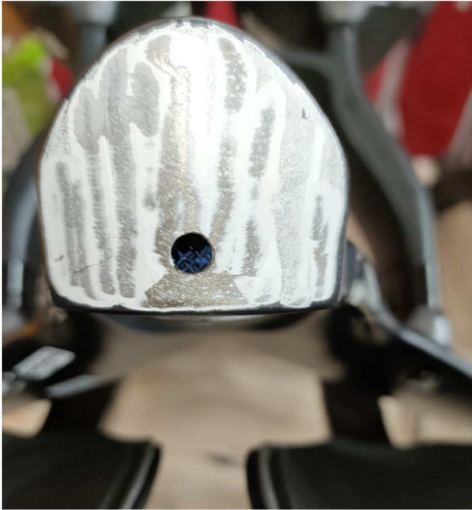
Figure 22 - Bar #2 oxidation inspection hole
