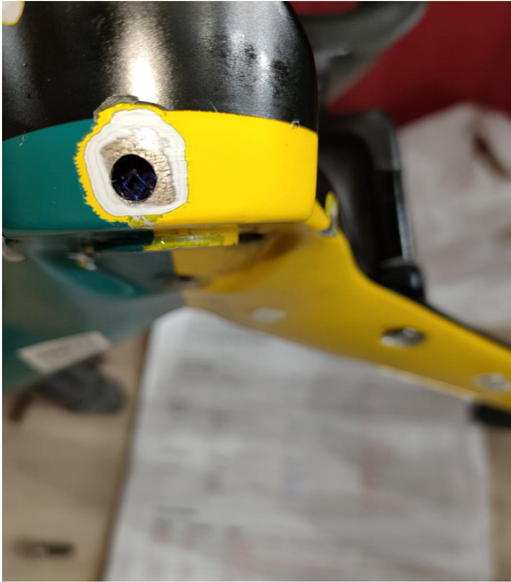
Figure 19 - Bar #1 oxidation inspection hole
