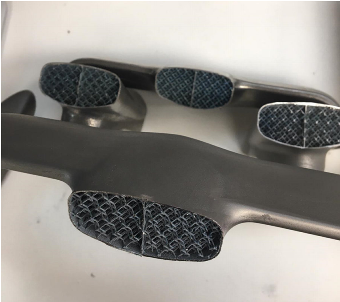
Figure 26 - Cut-through samples of Bastion Madison bars used as example of 'expected' level of oxidation (ref Bastion)
