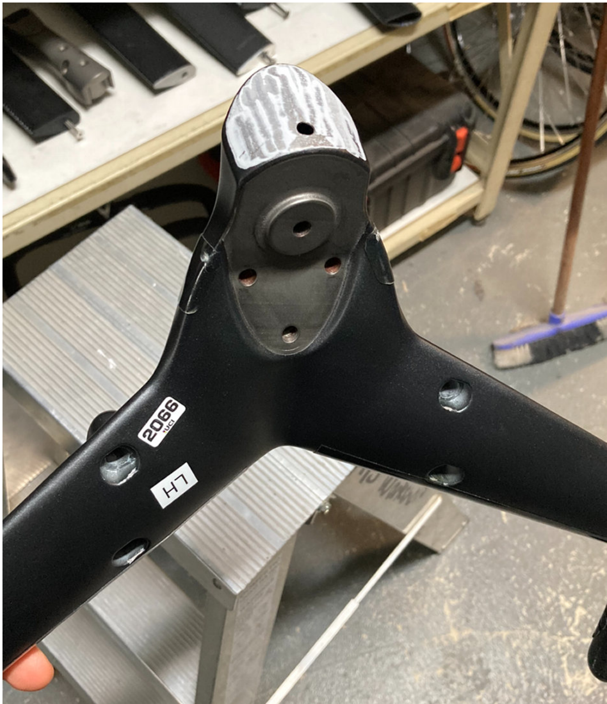
Figure 20 - Bar #2. Used by Leigh Howard in Tokyo. Note there appears to be beginning of crack forming at front of mounting face
