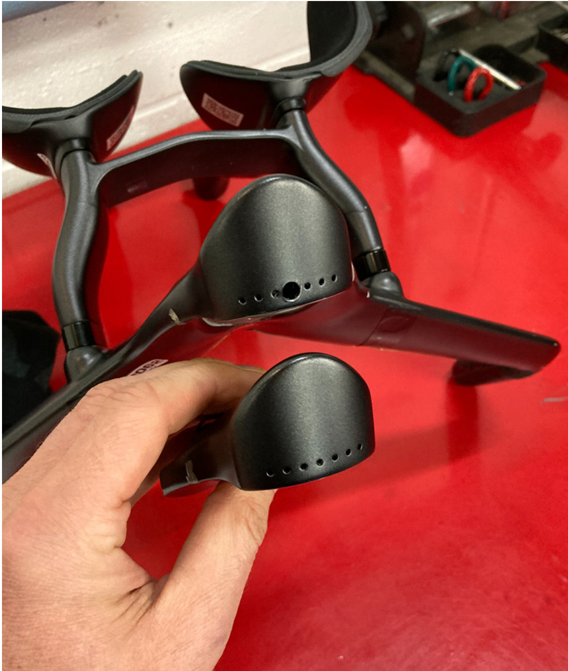
Figure 10 - Bars #3 (top) and #4 (bottom) showing presence of additional breather holes. Drilled hole in bar #3 by ACT to inspect oxidation. Bar #4 is that which failed under Alex Porter
