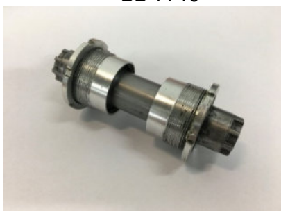
Figure 11: Comparison of Shimano Octalink Bottom Brackets
