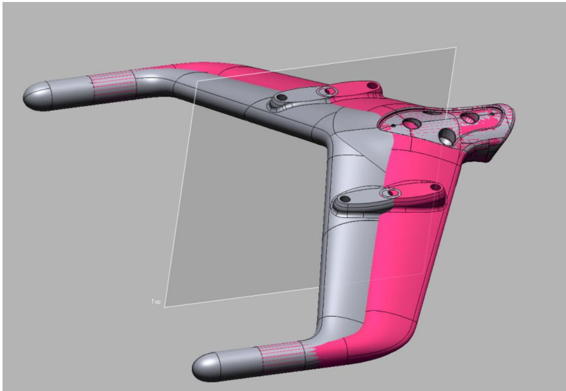
Figure 4 - Overlay of Argon18 standard pursuit base bar (pink) vs. Bastion CA06 design (grey)
