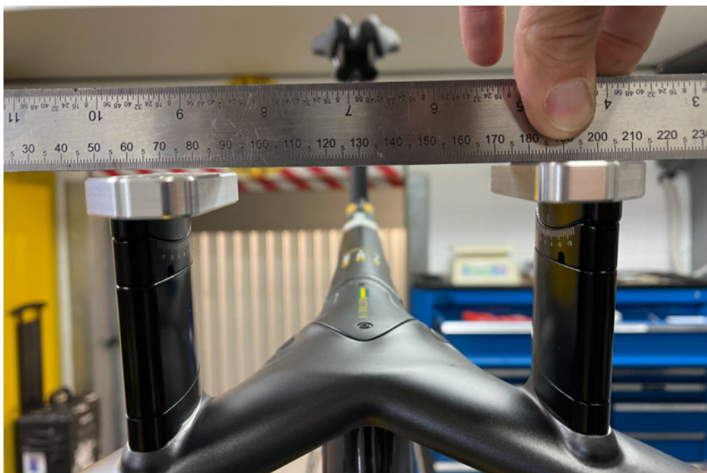
Figure 8 - Bastion bar #2 initial extension mounting surface issue
