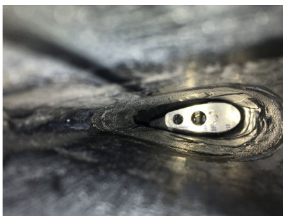
Figure 22: Correctly installed Seat Tube Plug in 2018 Frameset
