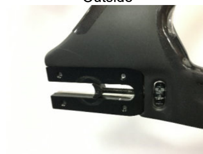
Figure 4: 2020 Dropout Plate Orientation
