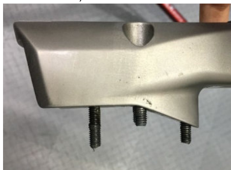
Figure 41: Adequate bolt length for 2018 Electron Pro
