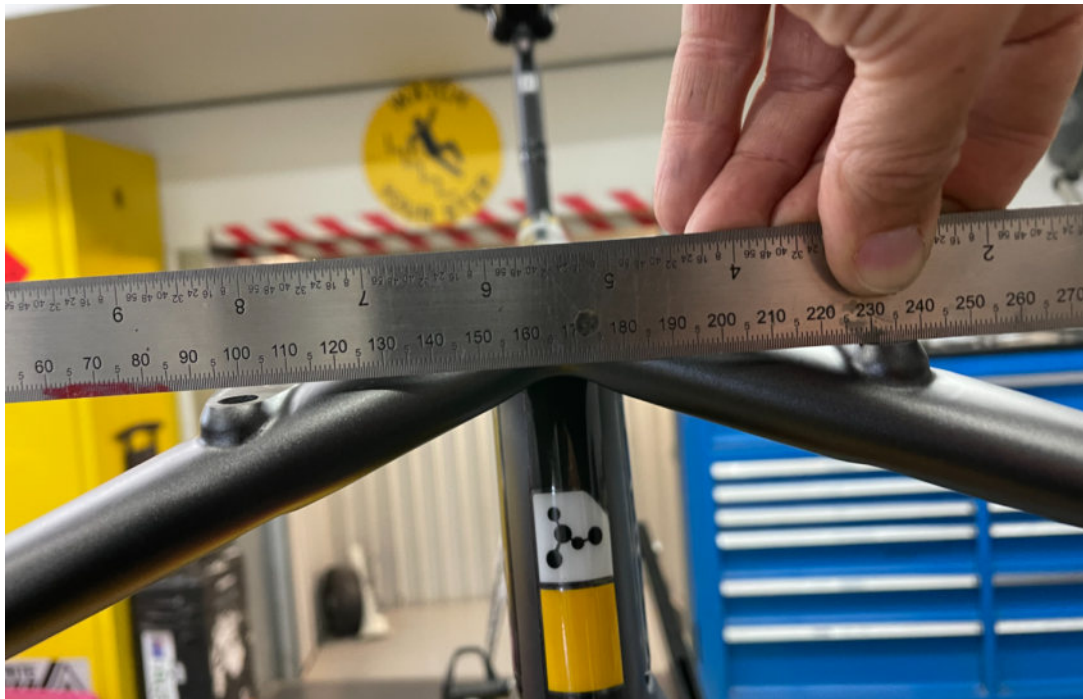
Figure 7 - Bastion bar #2 extension mounting surface issue
