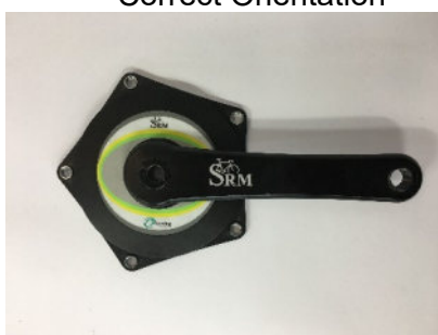
Figure 14: Correctly positioned and tightened SRM plate.
